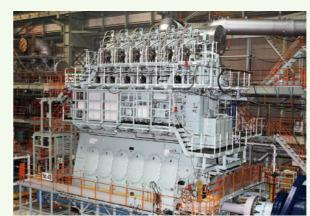
Electronically-controlled gas injection diesel engine (ME-GI)
