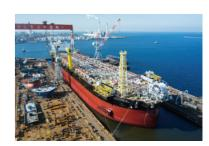
floating production storage and offloading system (FPSO for marine oil and gas
